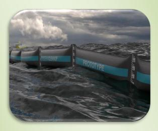
Slat's device floats along a coast and creates an artificial coastline, catching debris on the surface of the ocean. A connected conveyer then lifts the garbage into a central tower, where it is sorted for disposal.
