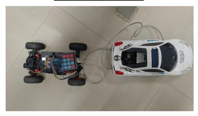
Data transfer from vehicle to vehicle through LI-FI, Transferring the message in traffic through head light to tail light of other vehicle. Data transmission time is 250 time faster than the Wi-Fi.
