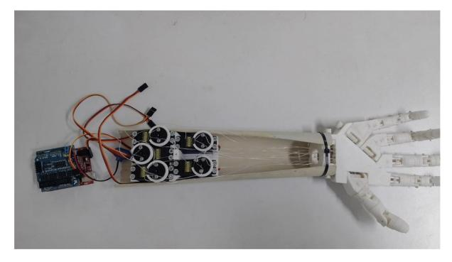
**Automated prosthetic hand**, which simulates the normal hand motion similar that of human hand. All the reflection action are given as a input to the robot hand ,through camera capture human action are recorded and same is simulated as input to the prosthetic hand.
