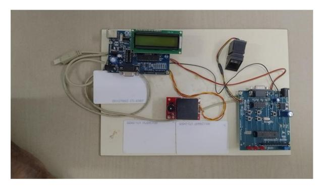
**Safe Optical Scan and Voting System** developed to carry out the voting in safe and protected manner preserving the citizen rights. The verification is done by checking all the aadhar details (iris checking, finger print checking and basic demographic details.) which allow them to cast their vote anywhere in any location.
